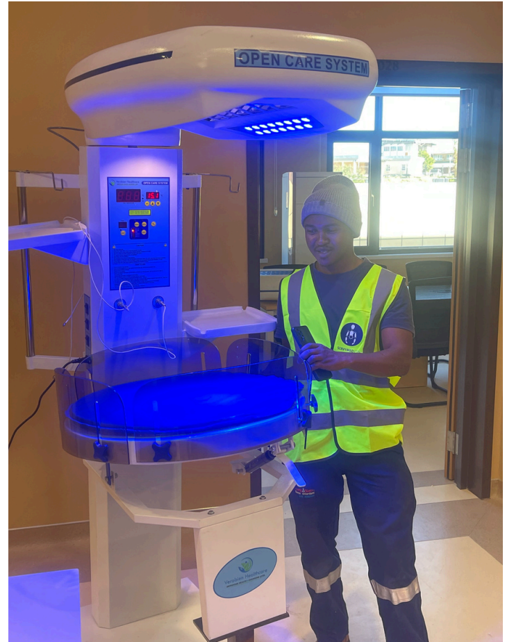
Ratanang, Monts'onyane, biomedical technician installing a neonatal baby warmer at Maseru District hospital. Photo by Mphatso Tsoka / PIH
